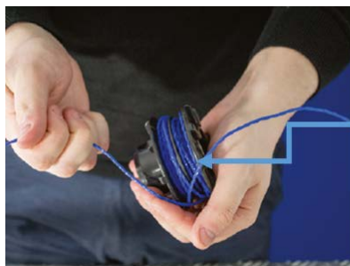
Wrap the nylon cord around the spool in an anti-clockwise direction until you have approximately - 150 mm (6").
