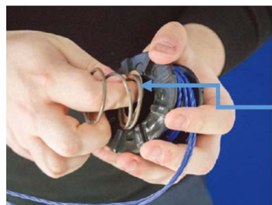
Reinsert the washer and spring into the spool. Once complete re-attach the spindle to the cutting head.
