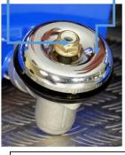
If spacer comes off it should be placed onto head cup side down
