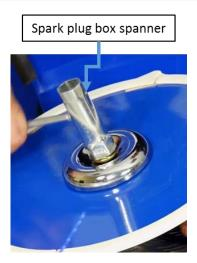
2.9. Attaching cutting assembly to drive shaft.
