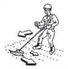
5.3.4. Keep cutting deck parallel with the ground. Do not tilt the nylon cutting or blade head during operation.
