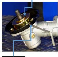
Allen key used to lock shaft
