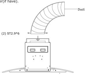
4. Align the hood body with the hood mounting bracket. Gently lower the hood until it securely engages the bracket.
