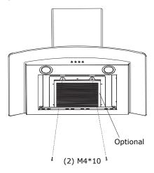
4. Install grease filter after charcoal filter is installed.
