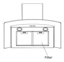
3. To install the charcoal filter, secure the square shape charcoal filter by two screws M4\*10.
