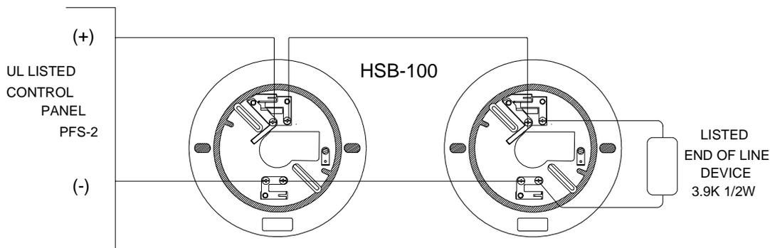
**Non polarized, not current limited. No annunciator output.**
