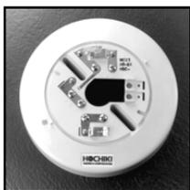
The HSB-100 Heat Detector Base Series is designed specifically for use with the HOCHIKI Rate of Rise Thermal Detector Model DSC-EA. The HSB-100 is a 6" diameter base that has no current limiting nor annunciator output features. A direct short occurs across the loop when the detector is actuated. Heat detectors are not recognized as proper detection for life safety protection, therefore they should be utilized only for the protection of property.
