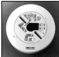
The HSC-L Heat Detector Base Series is designed specifically for use with the HOCHIKI Rate of Rise Thermal Detector Model DSC-EA. The HSC-L Series is a 6" base featuring a current limiting resistor, latching annunciator output and a latching circuit so the alarm LED will remain lit until the control panel has been reset. Heat detectors are not recognized as proper detection for life safety protection, therefore they should be utilized only for the protection of property.
